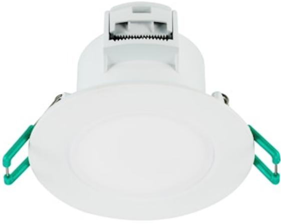
Integrated LED recessed spotlight, fixed, non dimmable, 3 CCT 2700K-3000K-4000K, 100° degree beam angle, polycarbonate white body, low profile 47mm recessed depth, IP65 from the front, IK03, loop-in/loop-out terminals for fast wiring, 87mm bezel diameter, 68-74mm cutout, frosted lens. Additional silver or black bezel can be ordered as accessory.
